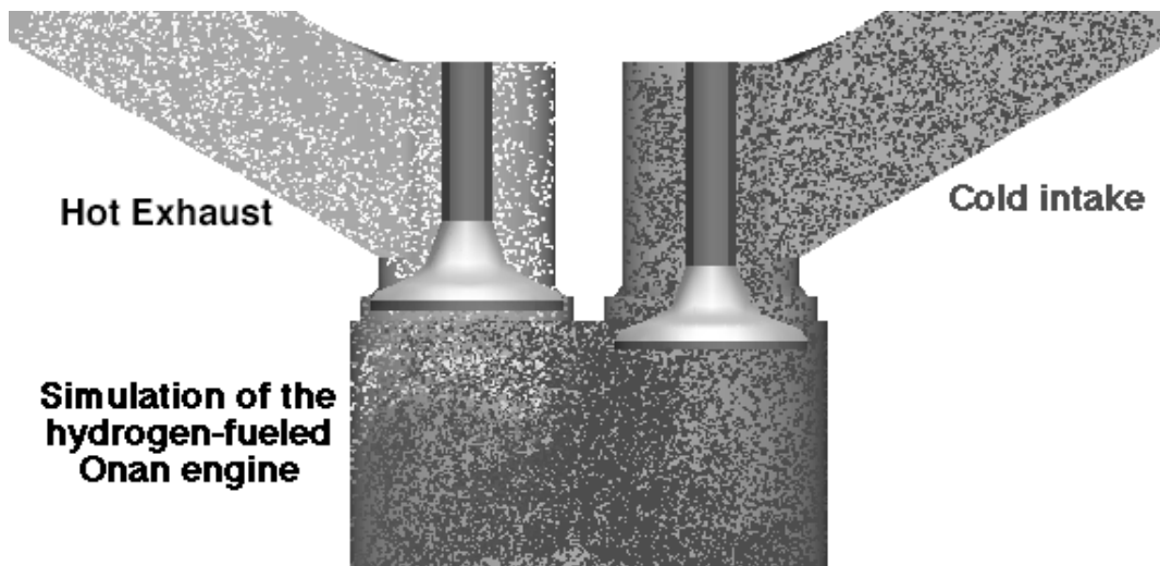
Fig. 1b. The intake flow at one time during the KIVA simulation. The cold air represented by the dark dots is compressing the hot residual gases, represented by the white dots. Note the exact rendering of the valve shapes and pockets.
