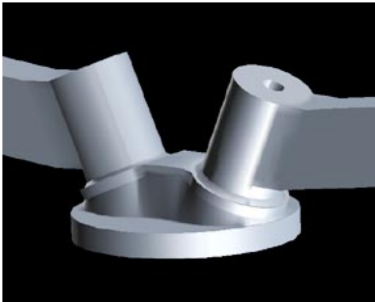
Fig. 11. An outside view of an angled-valve variation of the Onan engine. (Compare with Fig. 1.)
